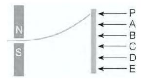
A beam of electrons is deflected in the magnetic field shown. The electrons that have passed through the field strike the screen at point P.
